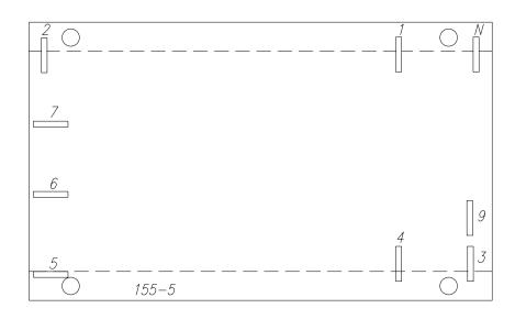
1: AC INPUT 2: AC INPUT 3: COUNT 4: RESET 5: OUTPUT PULSE AFTER 1-ST COUNT 6: OUTPUT T/W 7: OUTPUT B/W 8: N/A 9: COMMON
