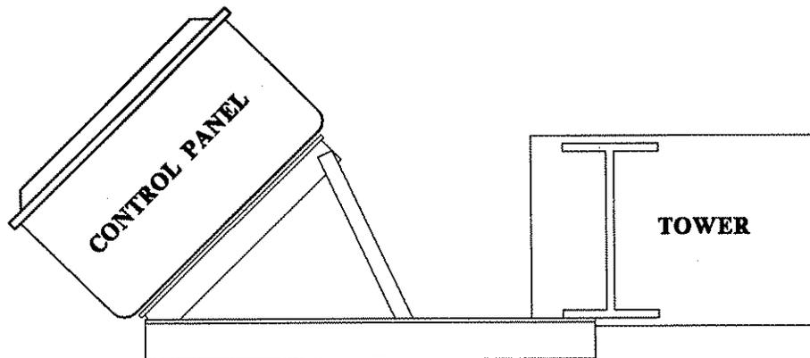
2. With the position bar (installed between upper angles), control panel can be rotated forward/to the side. (additional screw is attached to the tower's foot)
