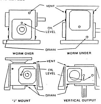
\*On double reduction units fill and vent each unit to levels shown.
