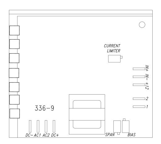
DC+: ARMATURE CONTROL AC1: AC INPUT AC2: AC INPUT DC-: ARMATURE CONTROL
