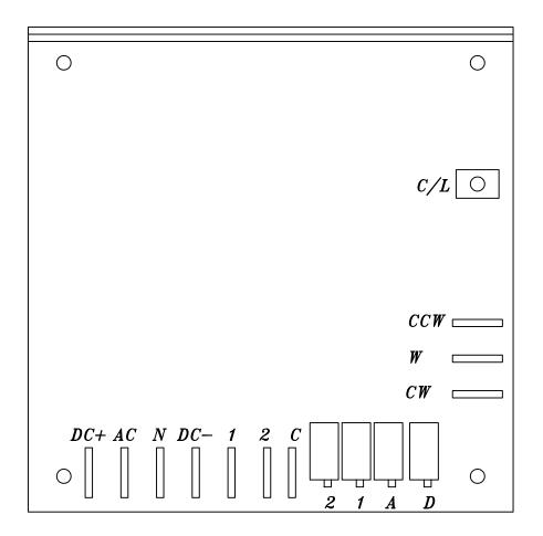
DC+: ARMATURE CONTROL. AC: AC INPUT – LINE. N: AC INPUT – NEUTRAL. DC-: ARMATURE CONTROL. 1: CONTROL – LINE. JOG SPEED 2: CONTROL – LINE. WRAP SPEED
