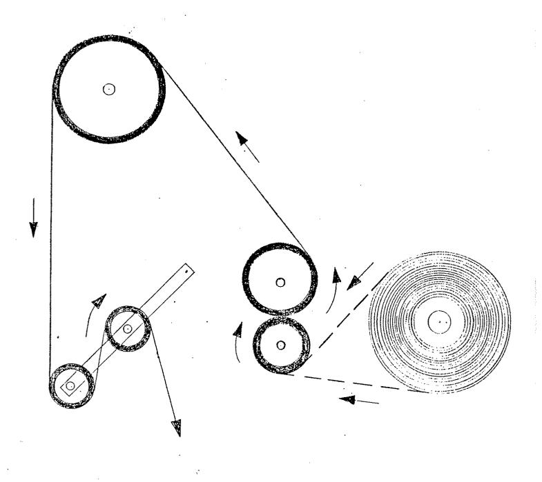
This diagram shows the pattern the film must take around the rollers for the proper operation of the stretchwrapper.
